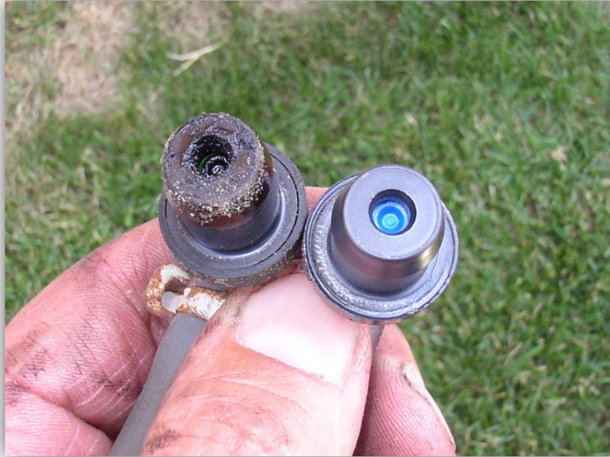
Figure 5: Comparison Between a Blocked PCV Valve and a Clean PCV Valve
